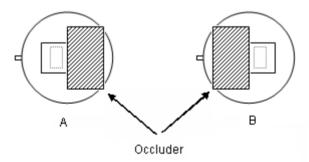
The sensitivity balance of sensor is calculated by measuring the sensitivity (signal output voltage) of each side and uses the formula as below:
